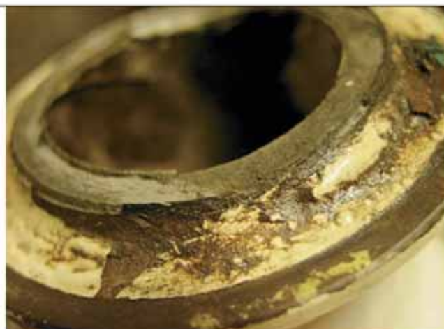
Photo n.5: general and pitting corrosion on the external surface of the axle, near the crack initiation region
