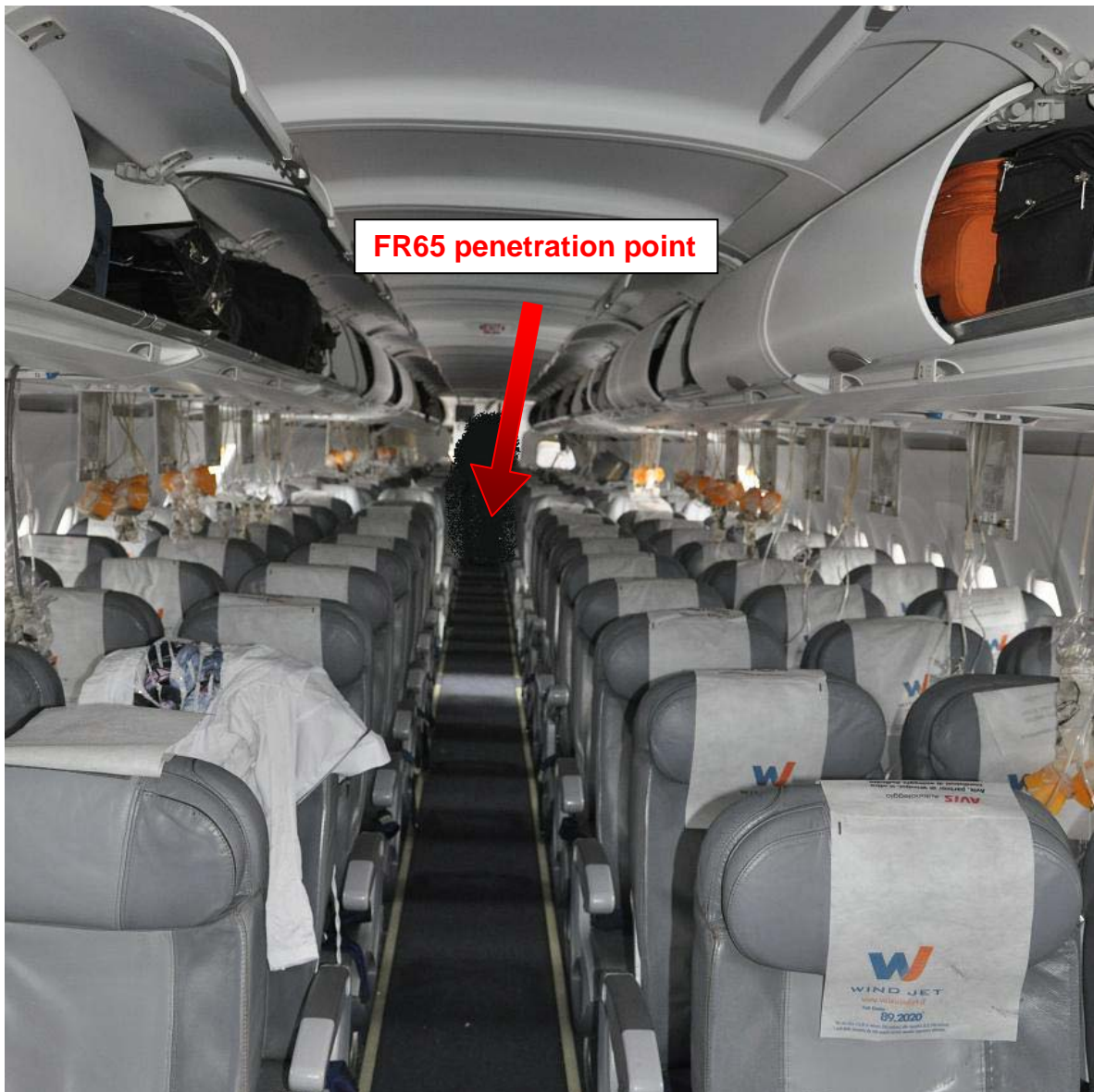
Picture 2: pax cabin condition after impact on the accident in subject.
