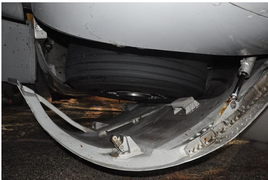
Picture 2: right main landing gear partially open.
