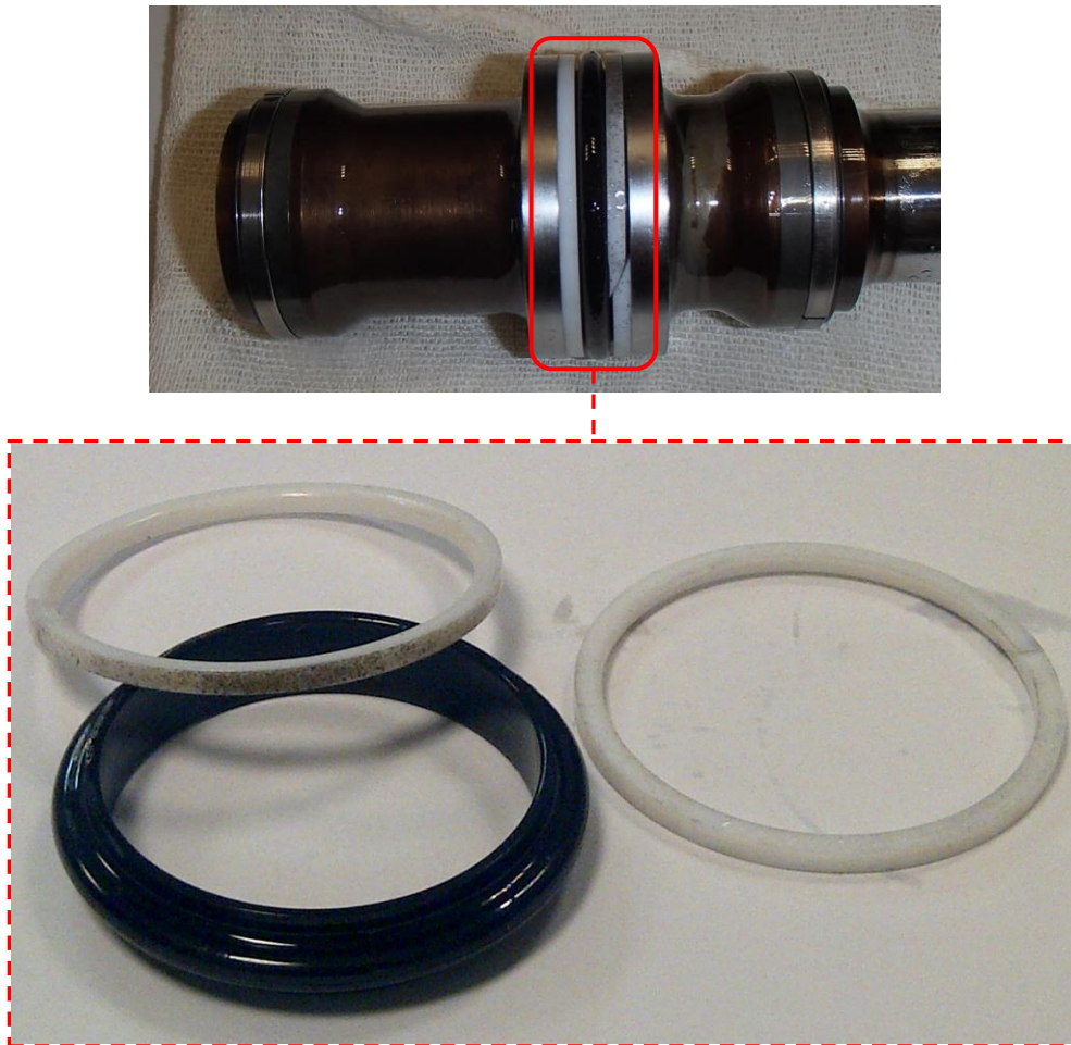
Picture 8: contamination found on LH MLG door actuator.
