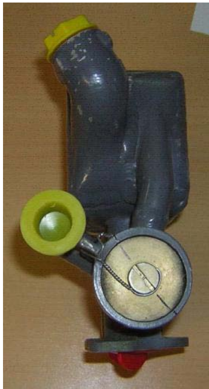
Picture 3: “oil to fuel heater”.
